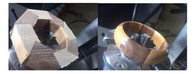
Once the inside is the same diameter I put the blank on a different step and simply turn it to final shape (just a bead). Sand and finish of your choice.
