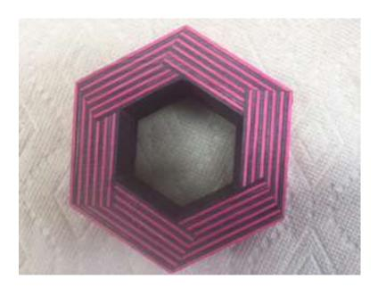
Once dry I cut the cylinder in about 1" thickness in preparation for turning.
